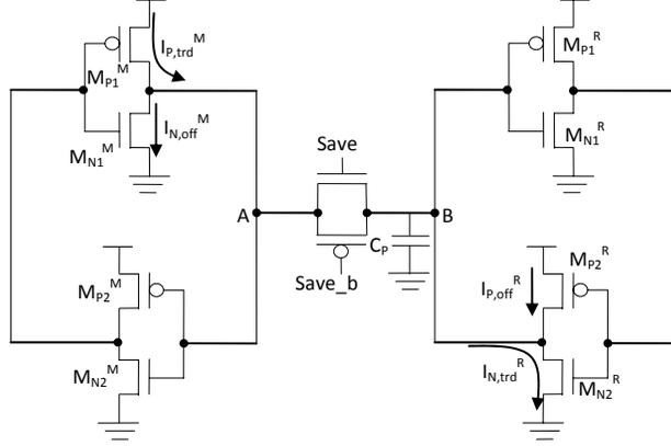
Fig. 1. Master and retention slave latch of RF
